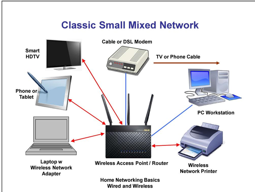
Above is the archetypical simple mixed wired and wireless network configuration diagram.
