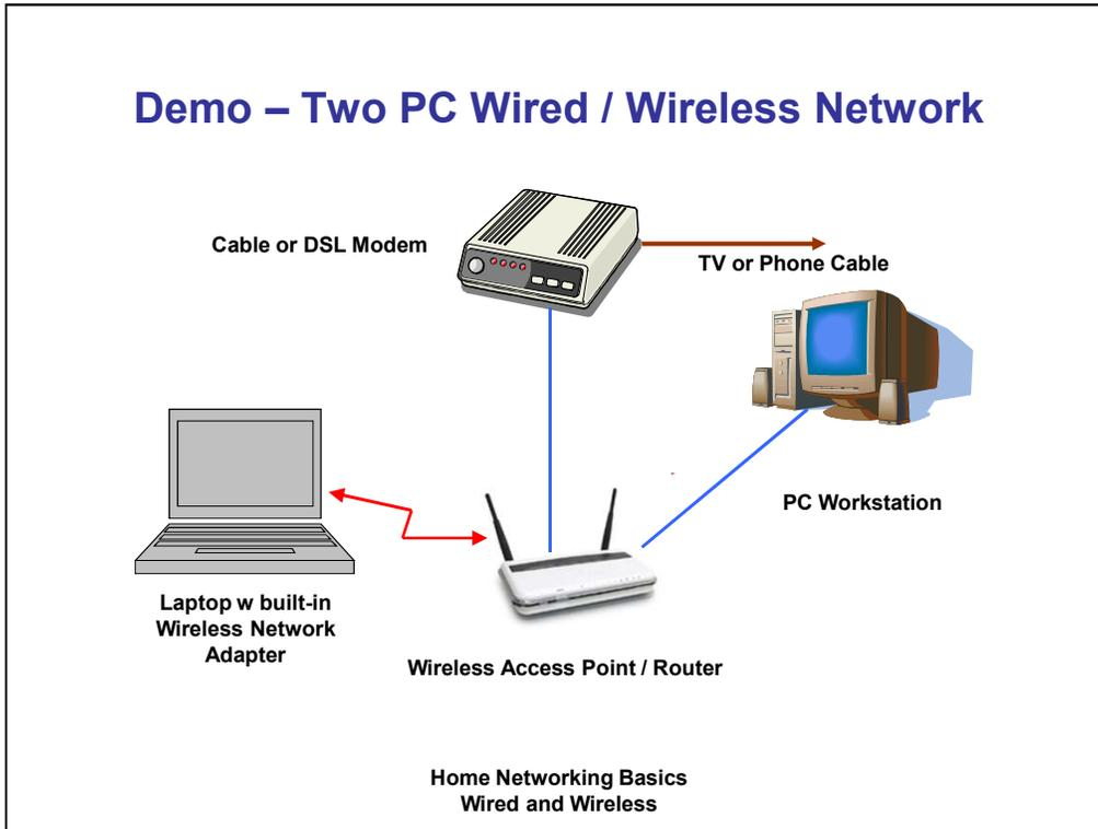
Above is a simplified two PC mixed wired and wireless network configuration diagram, a simpler version of what we reviewed above.
