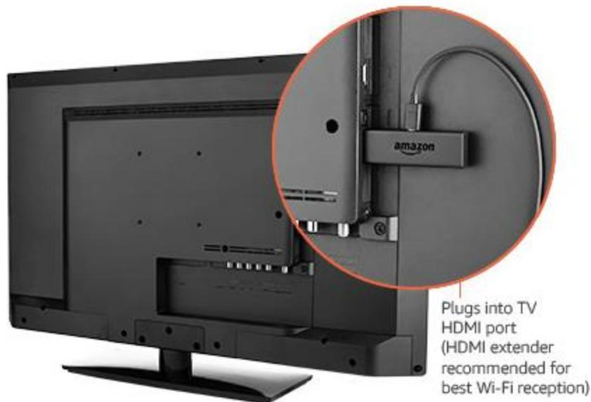
The package contains the Fire Stick itself, the remote, a HDMI extender cable, two AAA batteries and a power / adapter cord. The power cord has a micro USB jack on one end that plugs into the Fire Stick and a regular USB connector on the other end. The regular USB connector plugs into a USB socket on the small power adapter.
